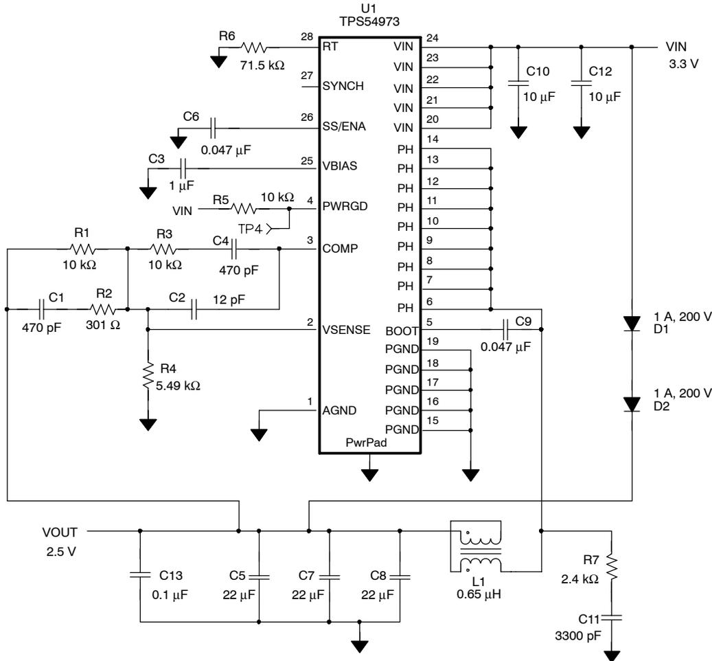
**Figure 9. Application Circuit**
